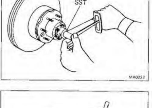
Loosen the adjusting nut until it can be turned by hand.
